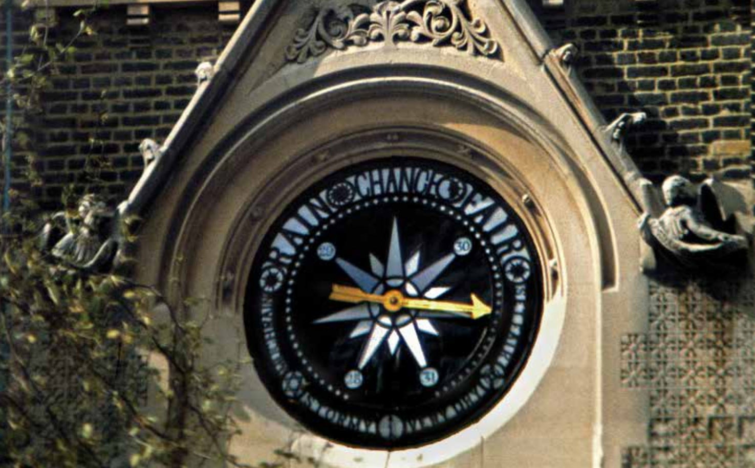
A turret barometer, the only one in England, on St Mark's Church, Dalston 1983. (Photo Alan Denney)
